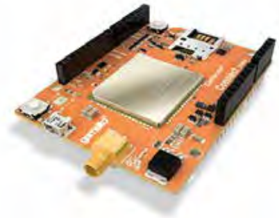
Gemalto's Cinterion Connect Shield adds cellular connectivity to an Arduino board.
