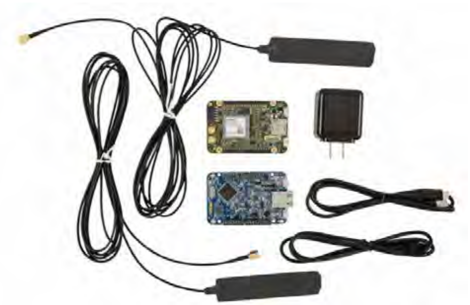
The AT&T IoT starter kit is based on the NXP FRDM K64F development board and includes an Avnet cellular shield, an AT&T LTE SIM card, two LTE antennas, two USB cables, an AC power adapter, and a microSD card.
