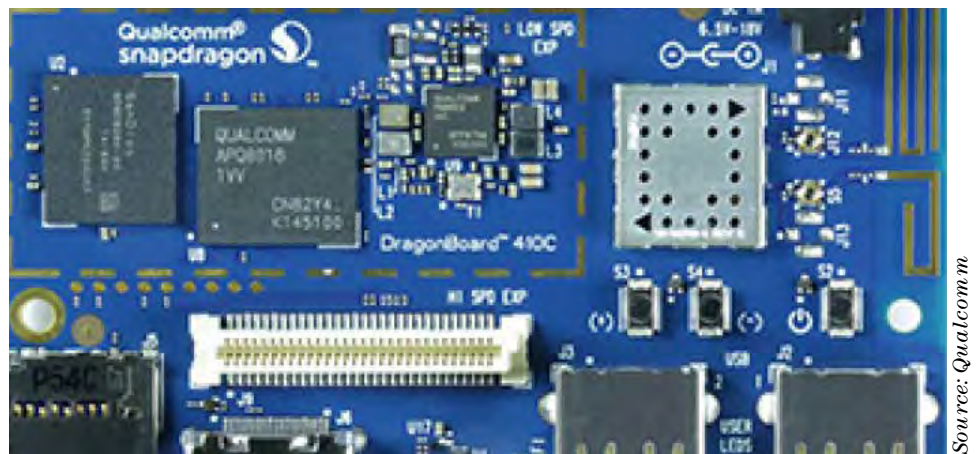
Qualcomm’s 410c development board enables a chip-down design using the 410E processor.
